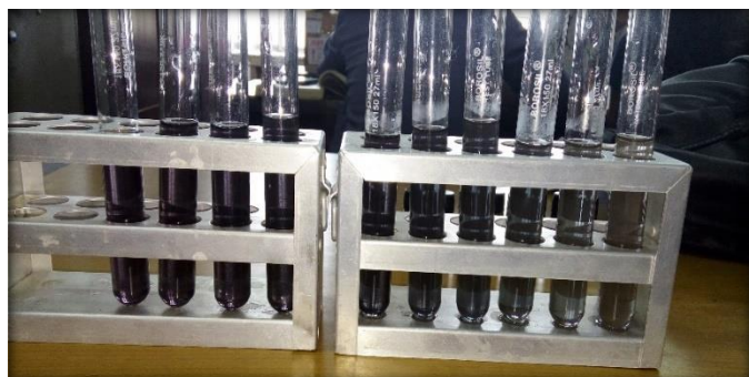
Fig. 1 Gradation of colour - formation of gold nanoparticles from 10%-100% at intervals of 10% seed extracts
